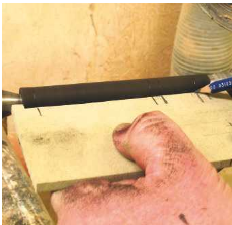
▲ Pic.22 Mark out the important details such as the spigots at the base and the one to go through the top, leaving enough waste at the finial end to allow for the hole left by the tailstock centre
